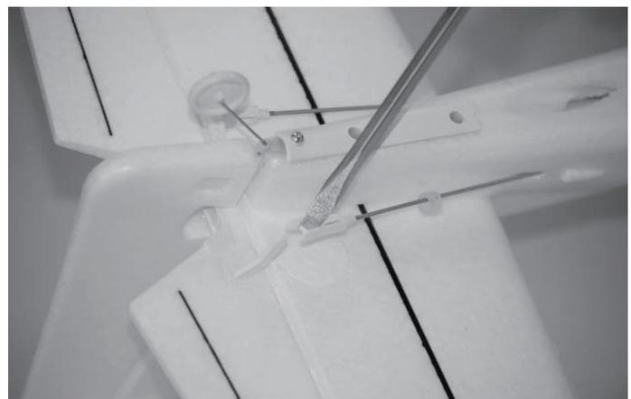
After connecting the clevises to the control horns view the vertical tail and rudder from directly above. The rudder should be 'in line' with the vertical tail when it's properly 'centered'. However, if the rudder is angled off to the right or left you can adjust the length/position of the pushrod/clevis so the surface is centered 'mechanically' while the trim lever on the transmitter is centered.
